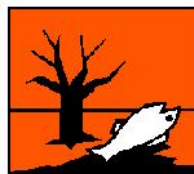
Dangerous for the environment (N)
